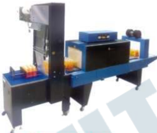
Automatic Shrink Wrapping Machine Model No. : MRE-SP-FA-14 Chamber Size : 2700 X 450 X 300mm Packing Speed : 15-20 packs/min. Power : 380V/50Hz - 20KW
