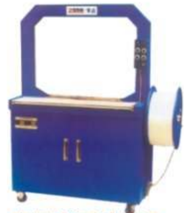
Automatic Strapping Machine Model No. : MRE-SM-FA-19 Packing Speed : 1.8 Sec./Strap Strip Width : 6-15mm Power : 220V/50Hz - 1.5KW
