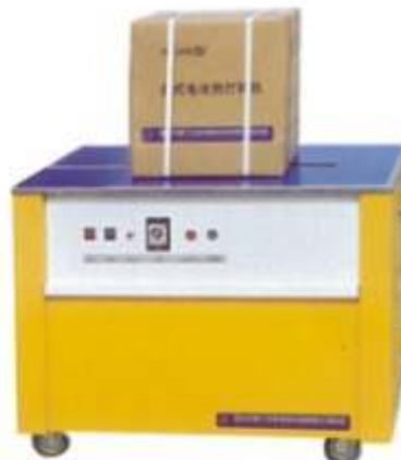
Strapping Machine Model No. : MRE-SM-SA-18 Packing Speed : 1.6 Sec./Strap Strip Width : 6-15mm Power : 220V/50Hz - 250W
