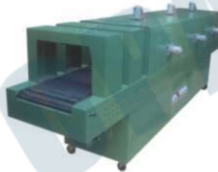
Shrink Packing Machine Model No. : MRE-SP-SA-15 Chamber Size : 2700 X 450 X 300mm Packing Speed : 4-10 packs/min. Power : 380V/50Hz - 18KW
