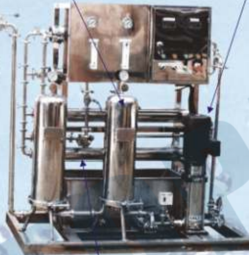
Reverse Osmosis System
