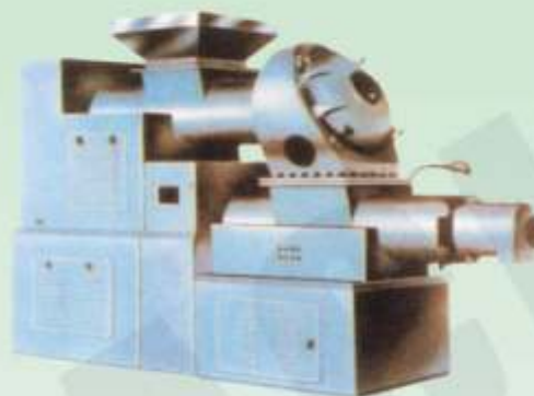
Soap Vacuum Extruder (Small Capacity)
